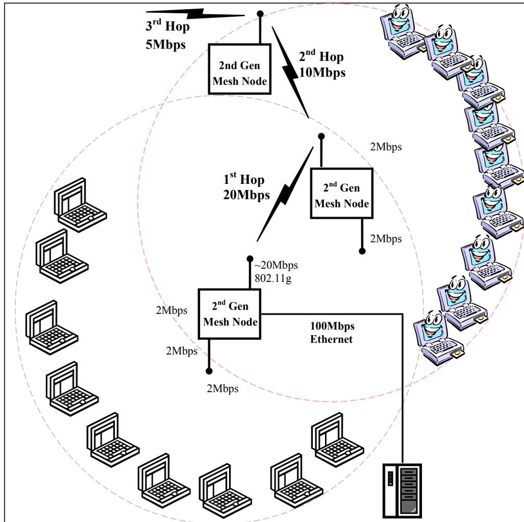
Figure 5: Second Generation Mesh Network
