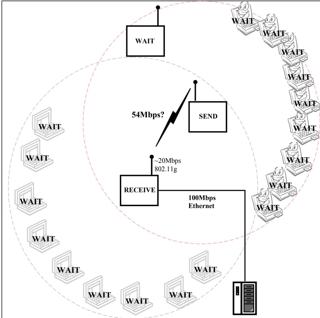
Figure 2: Radio must wait for every other radio in range
