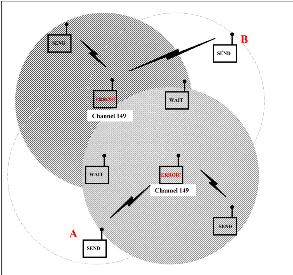
Figure 8: Hidden Node Problems in Second Generation Mesh
