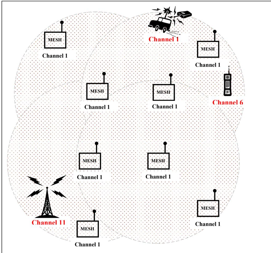
Figure 4: External Interference
