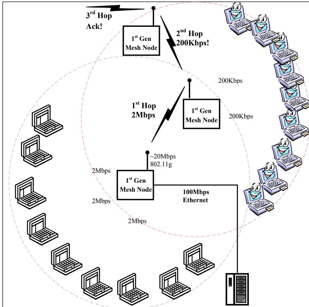
Figure 1: Sharing Client Services and Backhaul on One Radio
