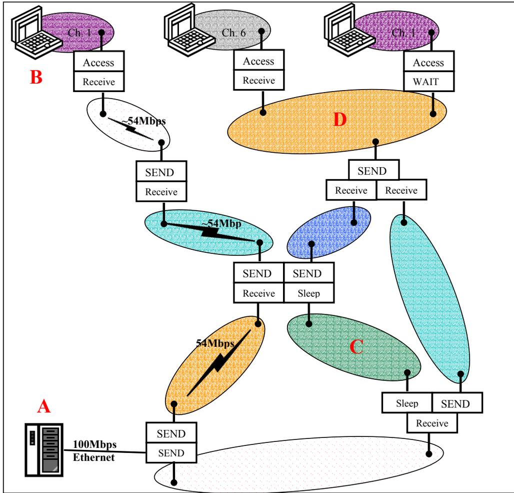
Figure 10: Multi-hop throughput in Third Generation Mesh
