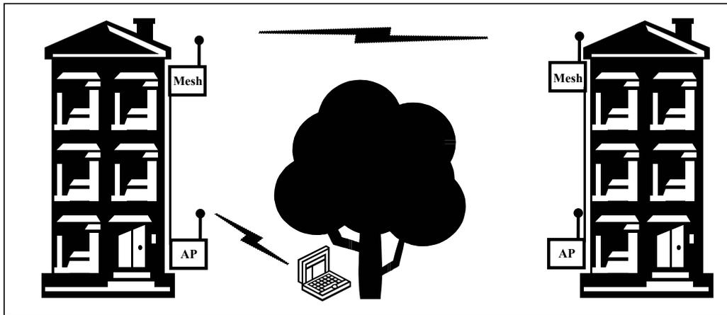
Figure 7: 1+1 Mesh solves antenna placement for clients and backhaul
