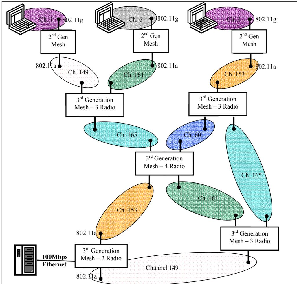
Figure 9: Third Generation Mesh Channel Use
