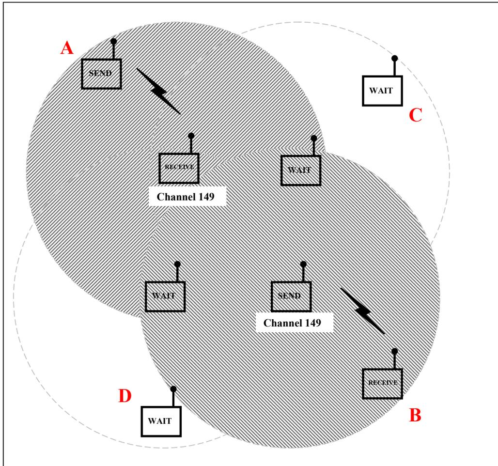
Figure 6: Backhaul Radio still must wait for every other radio in range
